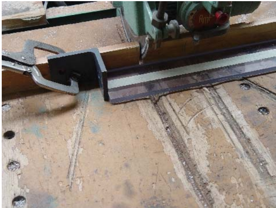
Coil mounting bracket components pieces being cut on a Radial Arm Saw
