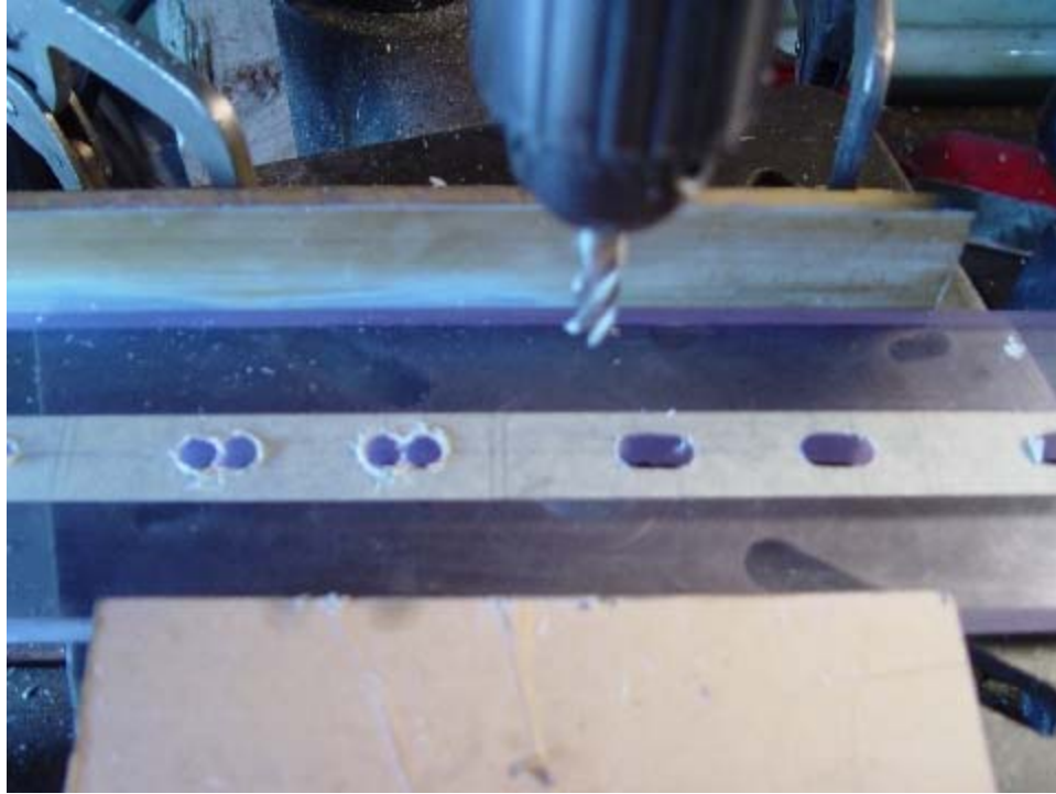
By using the stop as a guide, slide plexi back and forth to create adjustment slot
