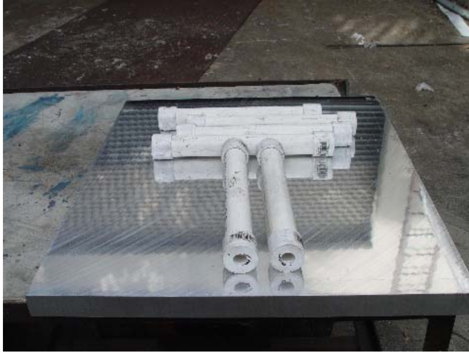
Clearance holes are drilled through the end caps
