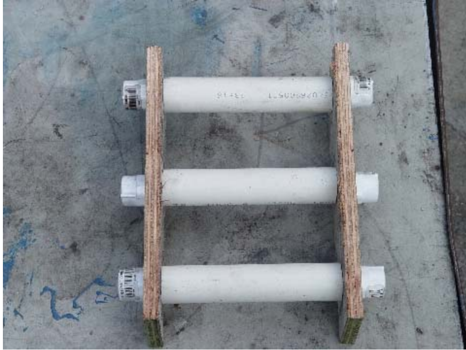
Mock-up illustrates how the sides are held together
