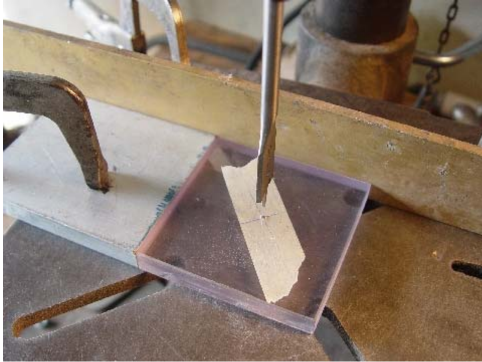
A stop block centers the rearward bracket component
