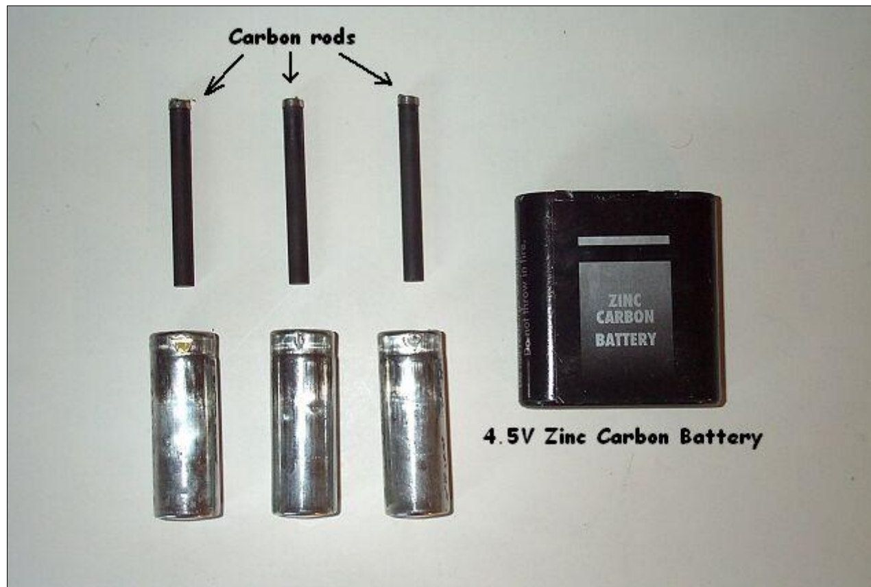
You will find the required carbon rods in any rectangular 4.5 V Zinc-Carbon battery.
