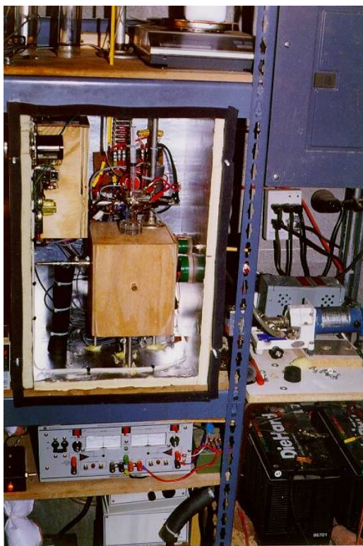
Figure 1.4. A calorimeter constructed by Edmund Storms, courtesy E. Storms. Note the DieHard® battery, lower right, that serves as an uninterruptible power supply. A power failure can ruin an experiment. Whenever possible, inexpensive, ordinary materials and instruments are used. However, experiments are never cheap, and they cannot be done on a shoestring.
