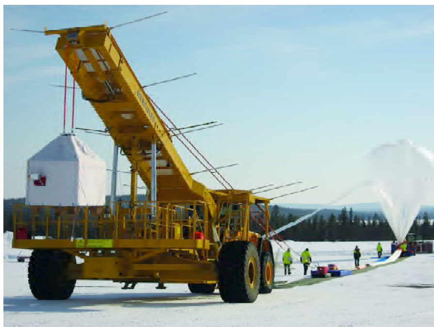
The BEXUS balloon gondola sitting on its transport vehicle with the stratospheric balloon in the background. The balloon has a total volume of 10 000 m 3 and grows to a diameter of 40 m when the maximum altitude is reached
