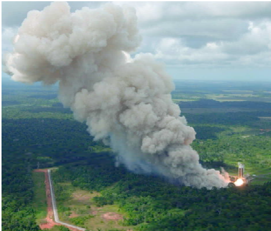
The P80 firing tests at the the Booster Test Stand at the Centre Spatial Guyanais in December 2007
