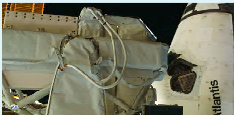
Mounted on Columbus, SOLAR is seen here in front of the Shuttle Atlantis, showing the movement bracket holding the scientific instruments (NASA)
