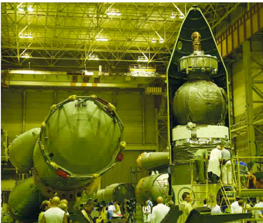
Top, Russian technicians lower YES2 onto the Foton-M3 spacecraft using a roof-mounted crane at the Baikonur Cosmodrome in Kazakhstan. Above, Foton-M3 is then placed inside the Soyuz rocket fairing, seen here alongside the Soyuz booster inside the Integration Building at Baikonur in September 2007
