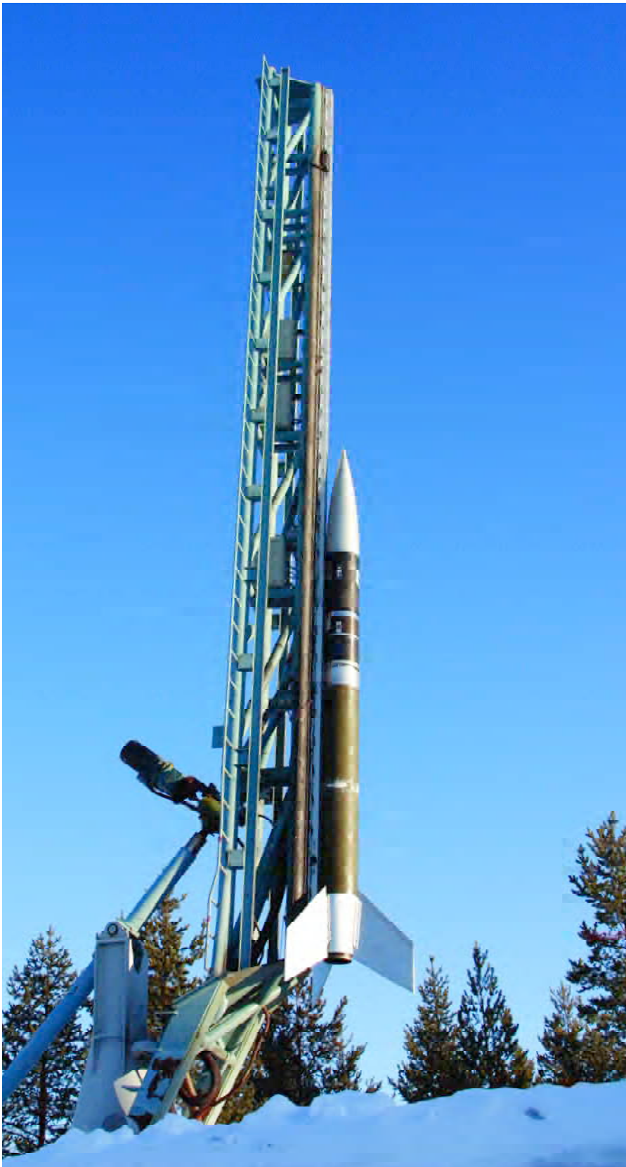
Used in the REXUS programme, the Improved Orion M112 is an unguided solid-propellant single-stage rocket, launched from Kiruna in Sweden
