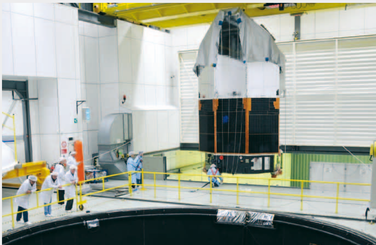
Herschel being lifted out of the Large Space Simulator at ESTEC after completion of its last TB/TV test
