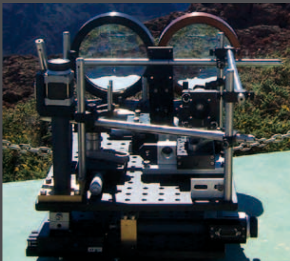
Transmitter telescope on La Palma looking towards the receiver on Tenerife. One of the large aperture lenses transmits single photons; the other receives the beacon laser from Tenerife for tracking purposes (Vienna Univ./MPQ)
