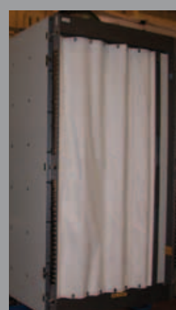
Extendable cubicle and privacy curtain on the WHC
