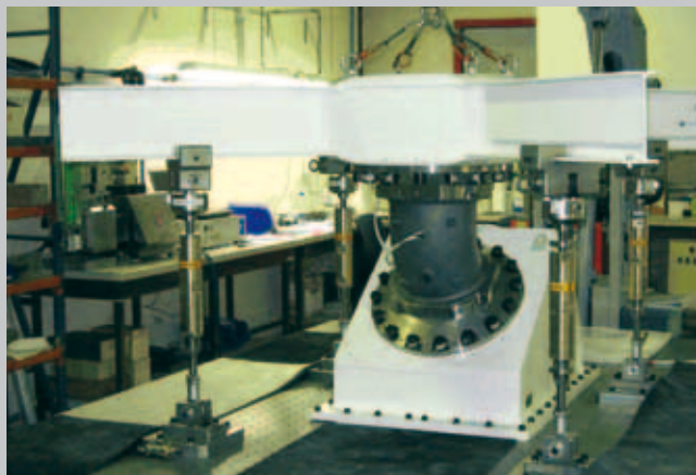
One of the silicon carbide-elements of the Gaia torus in preparation for its mechanical load testing
