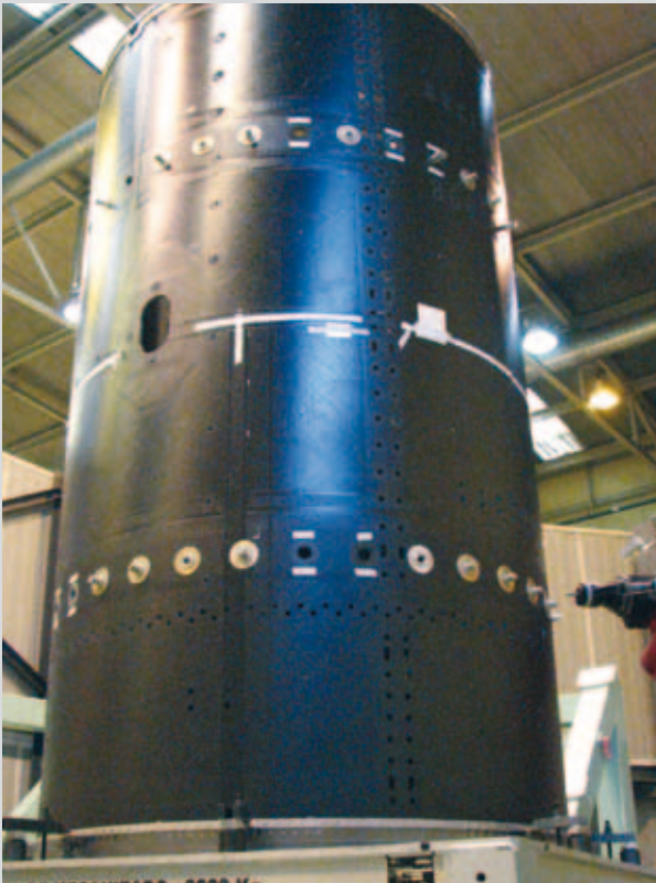
Alphasat central tube Protflight Model during manufacture (CASA)
