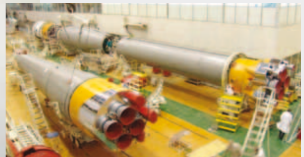
The first two Soyuz launcher stages ready in Samara
