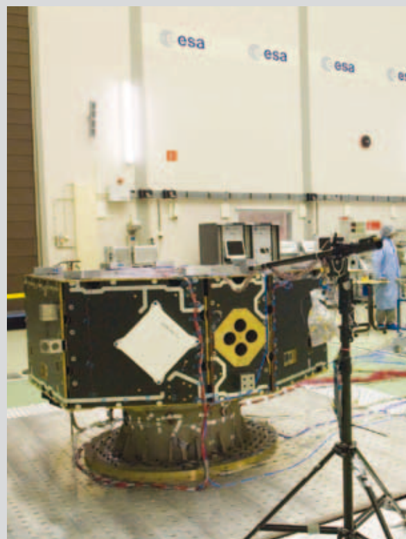
LISA Pathfinder science module during structural testing, on 'shaker' at ESTEC, Noordwijk
