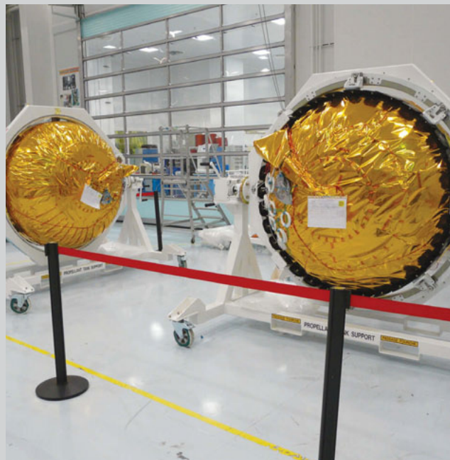
The large propellant tanks produced by MT Aerospace (Germany) shown ready to be integrated within the central tube of the Alphasat Service Module
