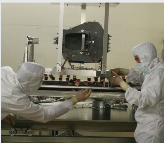
NIRSpec Flight Model camera optics during testing at cryogenic temperatures at the Centre Spatial de Liège, Belgium (CSL/Sagem Défense Sécurité)
