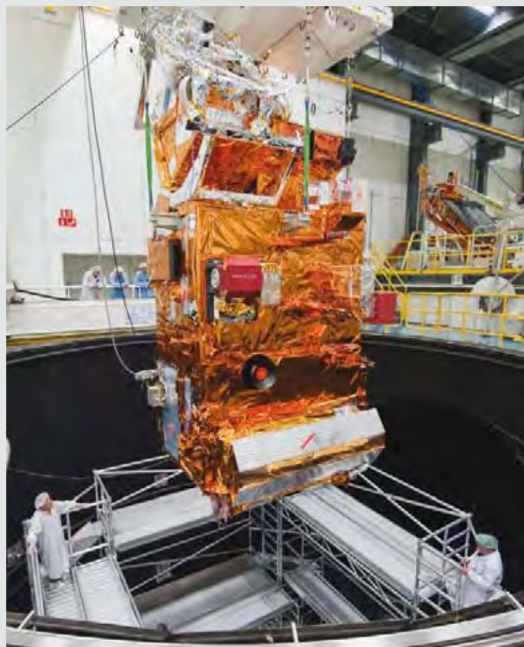
MetOp-B Payload Module being moved into the Large Space Simulator at ESTEC, Noordwijk
