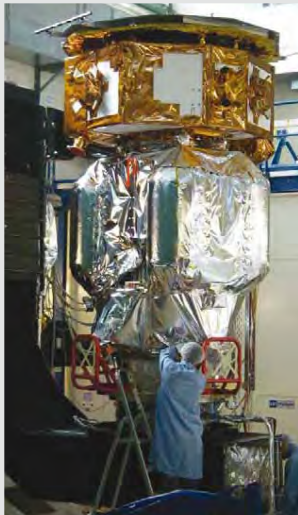
LISA Pathfinder in launch configuration after the Transfer Orbit Thermal Balance Test held at IABG. The Propulsion Module is the Flight Model, while the Science Module is partially made of Flight Models and thermal/structural dummies
