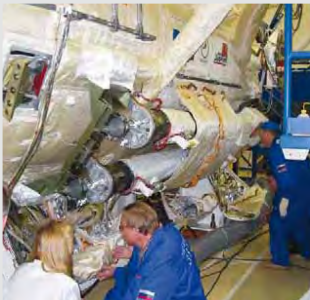
The European Robotic Arm spare elbow unit, before being covered under a thermal blanket, attached to Russian Mini Research Module 1 (MRM-1) for launch on the Space Shuttle Atlantis in May
