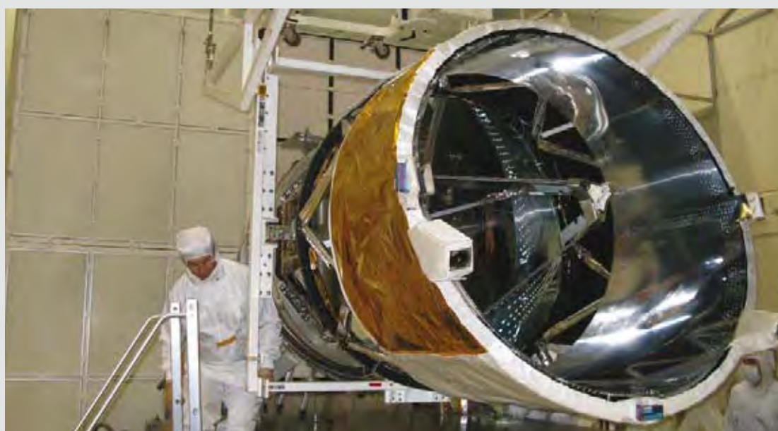
Aeolus telescope Flight Model during testing at the Centre Spatiale de Liege, Belgium (Astrium SAS)
