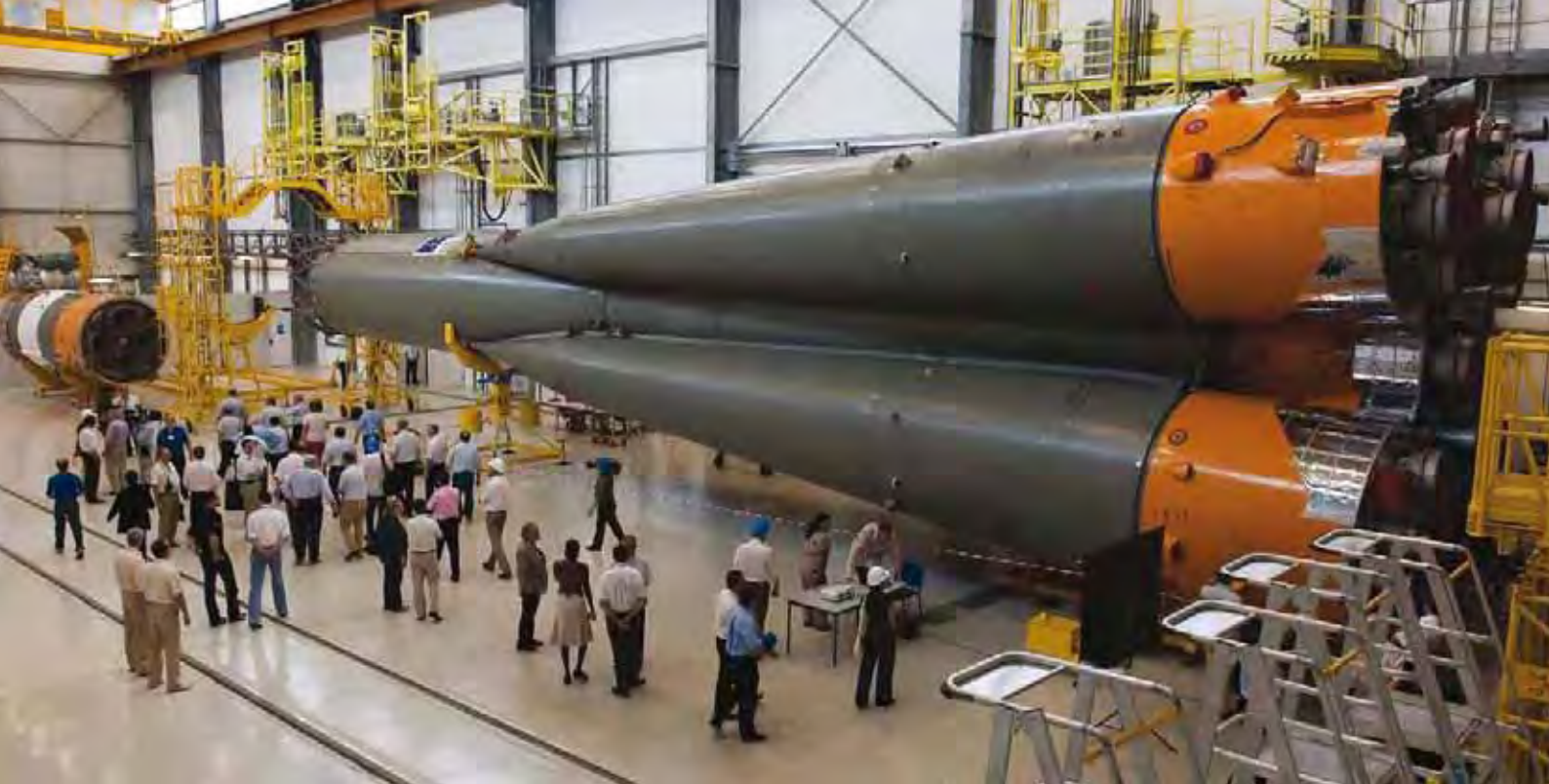
Integration of the first and second stages is complete for the first Soyuz to be launched from Europe's Spaceport in French Guiana ((ESA/CNES/Arianespace Optique Video CSG/P. Baudon)
