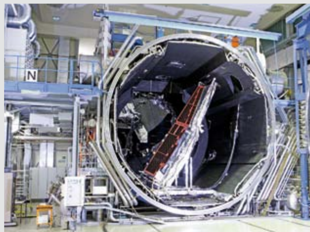
The first satellite of the Swarm constellation completed its thermal balance and vacuum test at the IABG test facility, Ottobrunn, Germany (Astrium GmbH)
