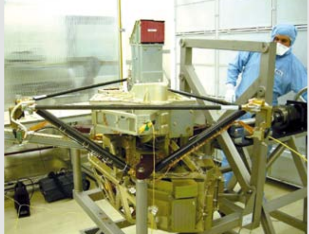
The fully integrated MIRI Flight Model on rotator table during its final inspection before covering with multi-layer insulation
