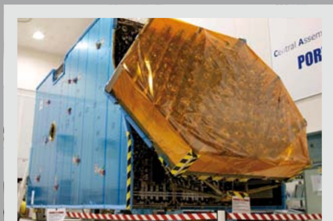
The Alphasat Repeater Module with integrated antenna feed at Portsmouth, UK, ready for shipment to Toulouse, France (Astrium Ltd)
