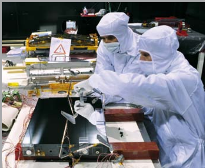
A Gaia mirror being prepared for integration on the Payload Module optical bench
