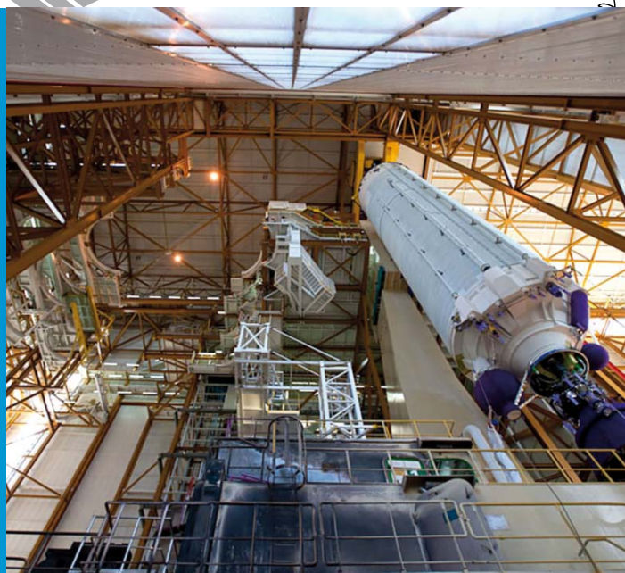
↑ The completion of initial build-up for the 200th Ariane: assembly of the Ariane 5 launcher (ESA/CNES/Arianespace Photo Optique Vidéo CSG)
