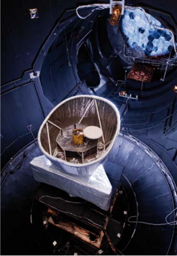
BepiColombo's Mercury Magnetospheric Orbiter and its sunshield in the Large Space Simulator at ESTEC, Noordwijk
