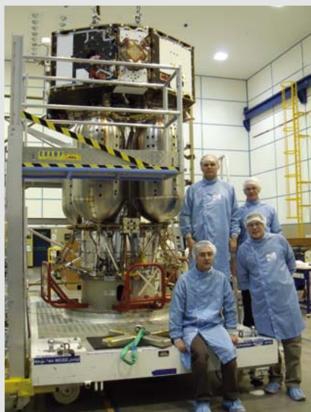
LISA Pathfinder Propulsion Module and Science Module Flight Models mated at the Astrium integration facilities, Stevenage, UK (Astrium Ltd)
