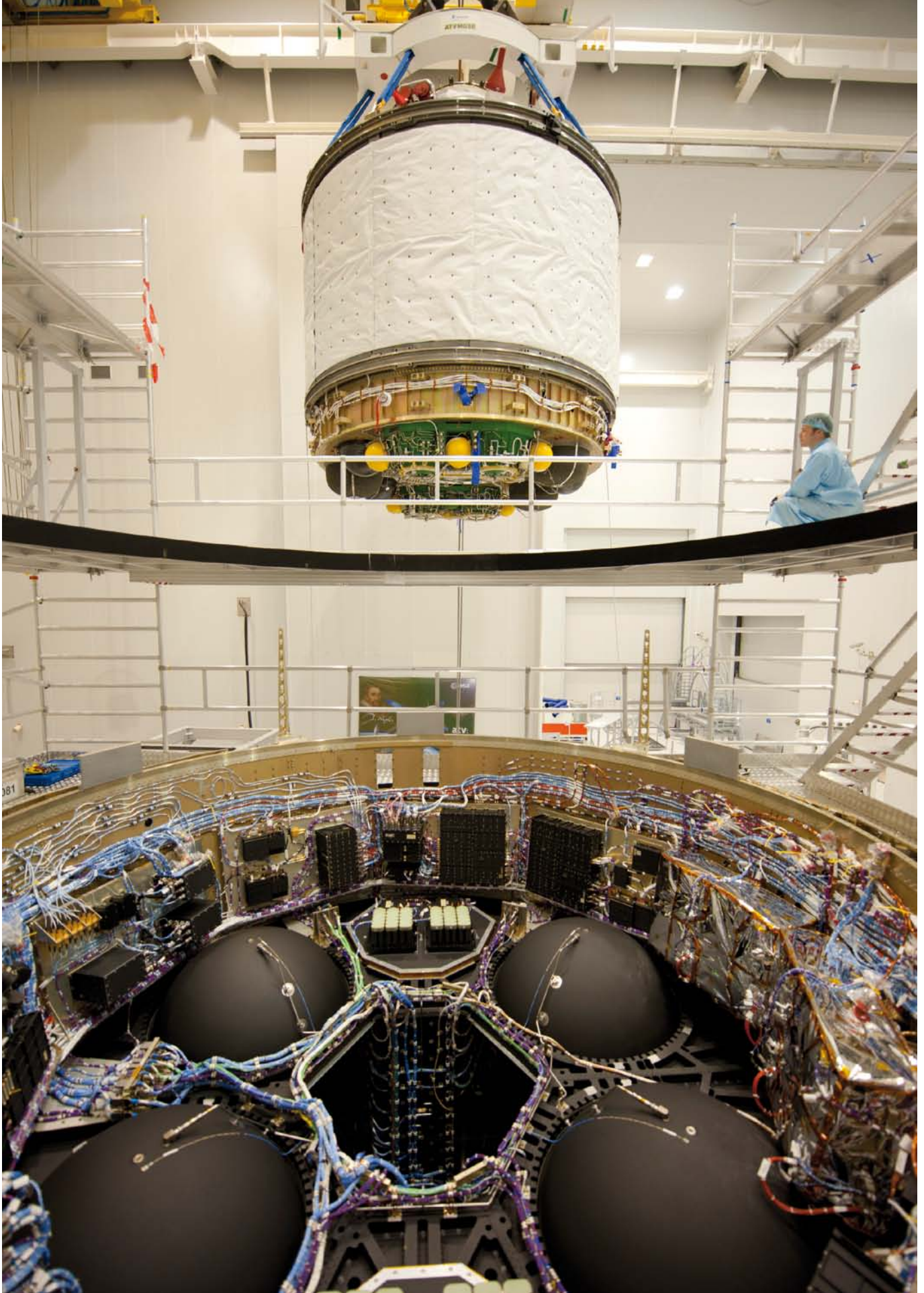
↑ ATV Johannes Kepler's Integrated Cargo Carrier ready for mating with the spacecraft's Propulsion Module, with the various tanks for fuel, water and gas cargoes visible
