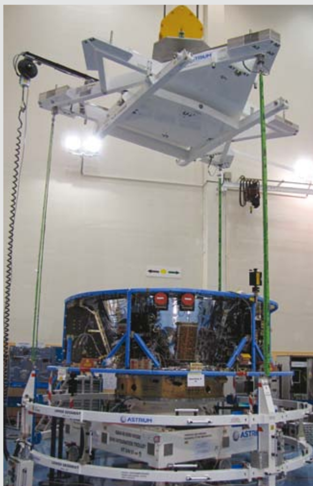
Gaia's Service Module ready to be weighed at the integration facility in Toulouse (Astrium)
