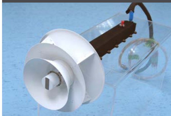
S-band TWT amplifier with an output power of 250 W in radiation-cooled design (TED)
