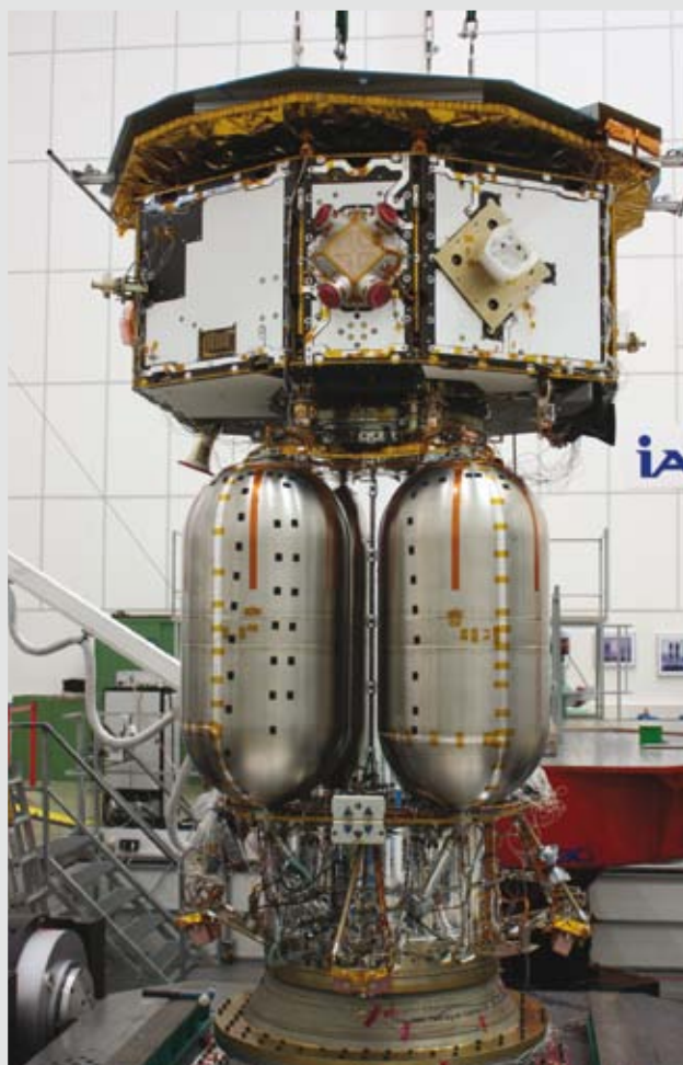
LISA Pathfinder Flight Model in launch configuration installed on the sine vibration shaker in Ottobrunn, Germany (IABG)
