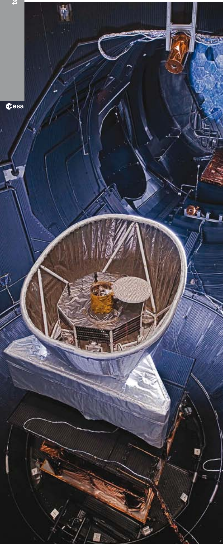
The MMO under test in the Large Space Simulator, free-spinning (above) and with its ESA-built sunshield (left)
