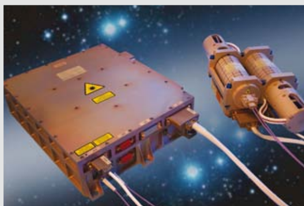
The last Swarm Absolute Scalar Magnetometers instrument with its sensor head (CNES/LETI)
