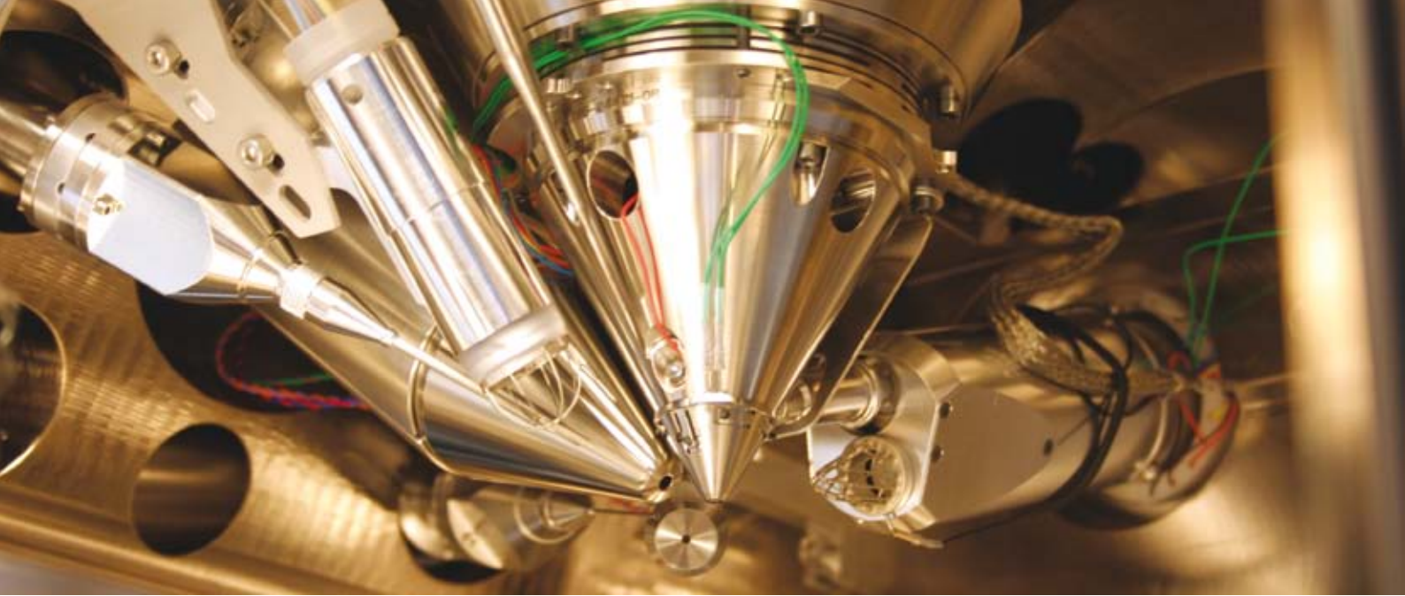
↑ A dual-beam focused-ion beam electron microscope, used for examining components to the exacting scales required
