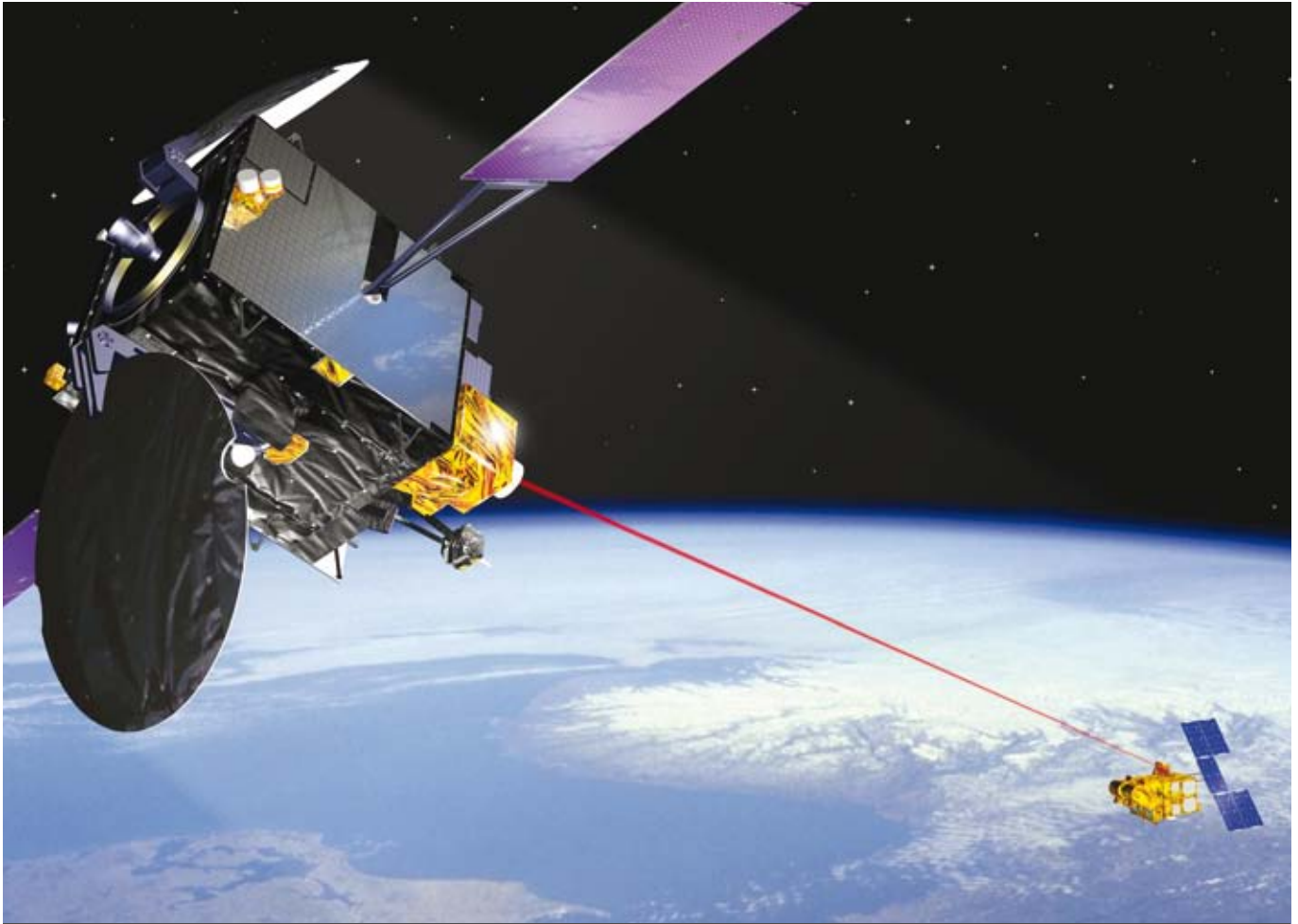
↑ On 30 November 2001, image data were transmitted for the first time by laser between two satellites. This was the spectacular demonstration of the SILEX (Semiconductor Intersatellite Link Experiment) system, where an optical link was established between Artemis in geostationary orbit and the French space agency's SPOT 4 in a low Earth orbit
