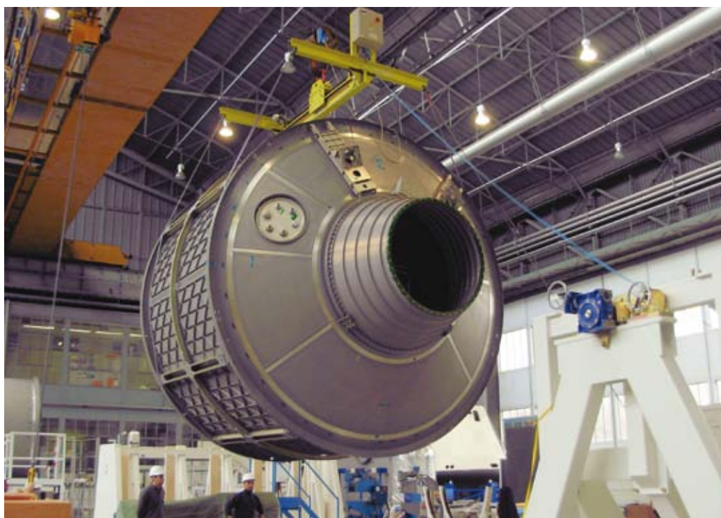
The pressurised module of ATV Albert Einstein seen during manufacture in December 2010 in Turin (Thales Alenia Space)
