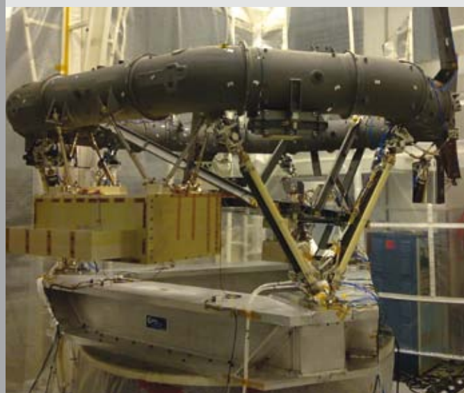
Gaia's PLM during the mechanical qualification tests at Intespace Toulouse (Astrum SAS)
