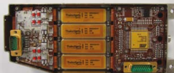
Sentinel-1 Electronic Front-end Qualification Model (Thales Alenia Space)
