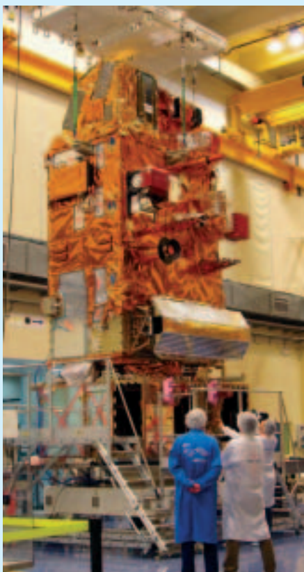
The MetOp-2 satellite during coupling of the Payload and Service Modules at EADS Astrium in Toulouse (F)
