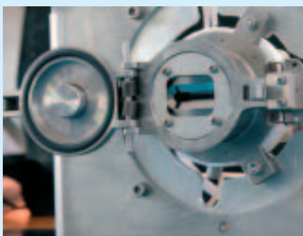
FEPP-8, an 8mm slit field-emission thruster for the LISA Pathfinder mission
