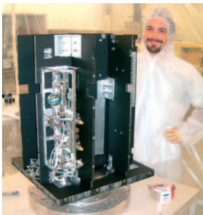
SSETI student Jörg Schaefer shows the student satellite's propulsion management system in the clean room
