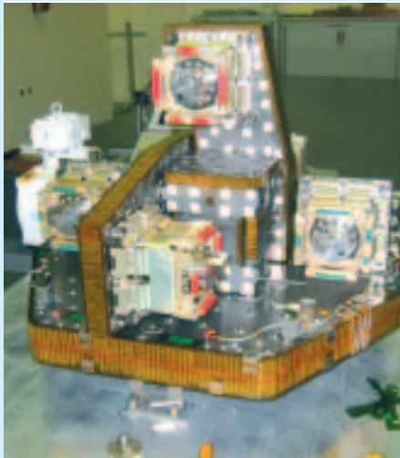
GOCE Gradiometer structural thermal model's core
