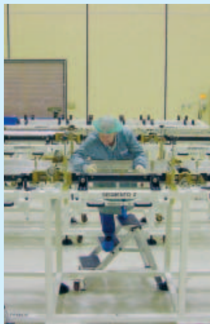
Integration of the arms for the SMOS structural model at EADS CASA
