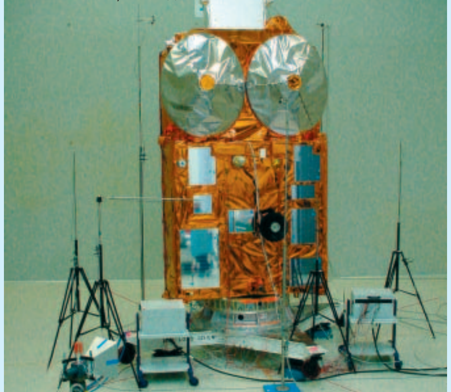
The CryoSat satellite after completion of the acoustic test in the dedicated IABG facility in Ottobrunn (D)
