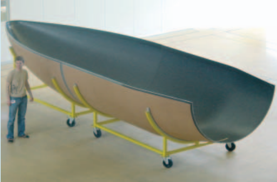
The Vega fairing (courtesy of Contraves Space)
