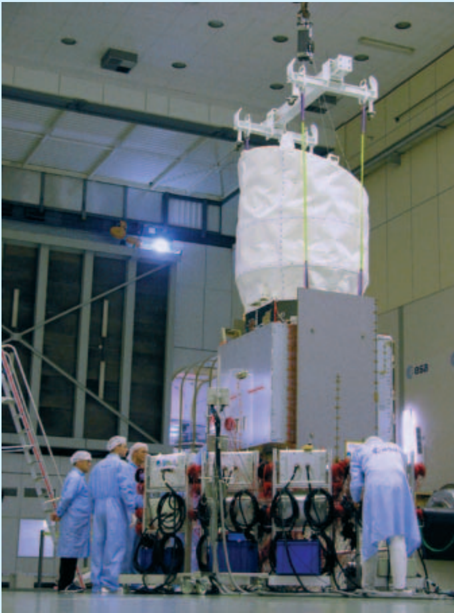
Structural model of Aeolus mounted on the multi-shaker in the ESTEC Test Centre in Noordwijk (NL)
