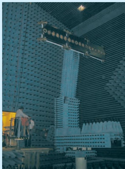
SMOS antenna arm mounted in the Antenna Test Facility at the Technical University of Denmark
