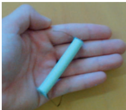
Prototype of a linear Electro-Active Polymer (EAP) actuator
