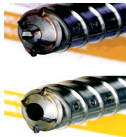
The Pasteur payload's drill-bit design concept. The drill's full 2 m extension is achieved by assembling four sections (one drill tool rod, with an internal shutter and sample-collection capability, plus three extension rods). The drill will also be equipped with an IR spectrometer for mineralogy studies inside the borehole. (Galileo Avionica)
