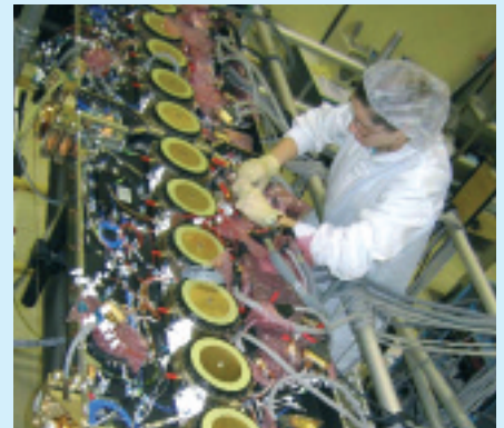
Integration of the SMOS protoflight model arm at EADS Casa Espacio
