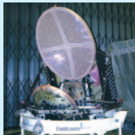
The Planck Flight Model telescope equipped with videogrammetry targets and protective covers on its support stand
