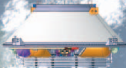
Ariane's payload adapter outfitting as the ConeXpress free-flying spacecraft
