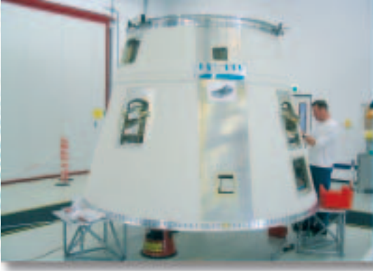
The Structural Model of Interstage-1/2 at Dutch Space in Leiden (NL) during integration. The interstage remains attached to stage-1 and carries six forward-facing solid-propellant retrorockets to ease separation at the end of the 107-second P80 burn. The interstage qualification tests are under way.
