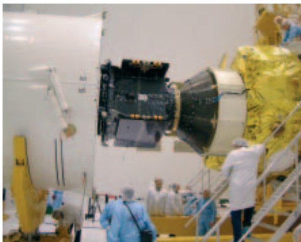
Encapsulation in the Soyuz fairing
