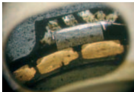
Over-worn brush on ASCAT's antenna deployment motor (left, arrowed). Normal wear on a bedded-in brush (right)
