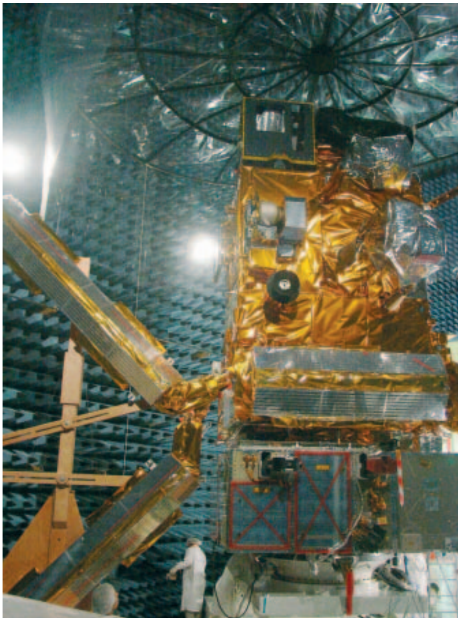
Checking the radio emissions of MetOp in the anechoic chamber in Intespace. The satellite's complex payload and many antennas made it difficult to avoid interference
