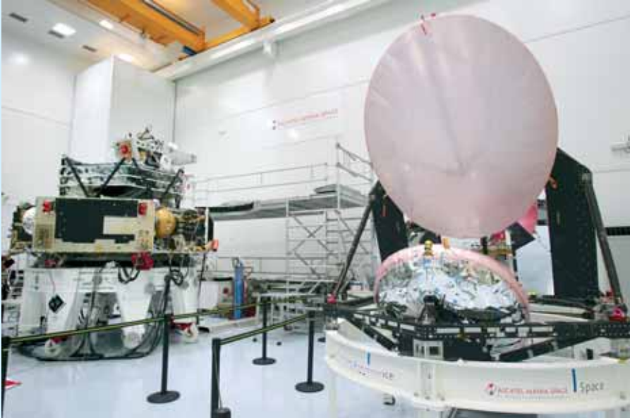
The Planck Flight Model: the telescope in front and the spacecraft at the back, in the final stages of integration
