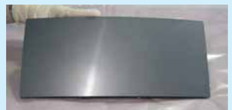
The optical face of the first FM secondary mirror blank for Gaia. The optical surface accuracy of better than 50 µm rms will be improved by polishing to better than 10 nm rms
