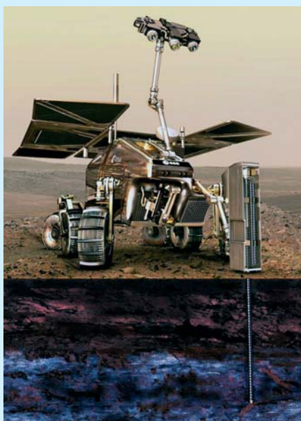
The Pasteur instrument exobiology payload on ExoMars will include a drill that will be able to look for traces of life forms beneath the surface of Mars
