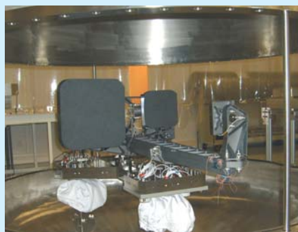
Qualification Model of JWST's NIRSpec FORE three-mirror anastigmat
