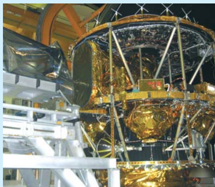
Left: MSG-4 in optical vacuum test configuration at Thales Alenia Space, Cannes (F). This test demonstrates the performance of the SEVIRI infrared channels, with the detectors operating at temperatures of 85K to 95K
