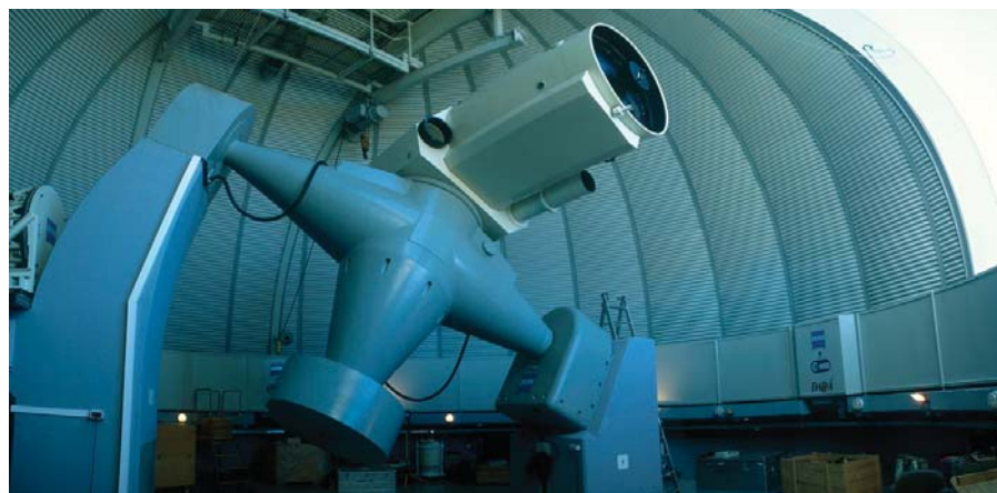
The 1 m Zeiss telescope, with its 'English' equatorial mount
