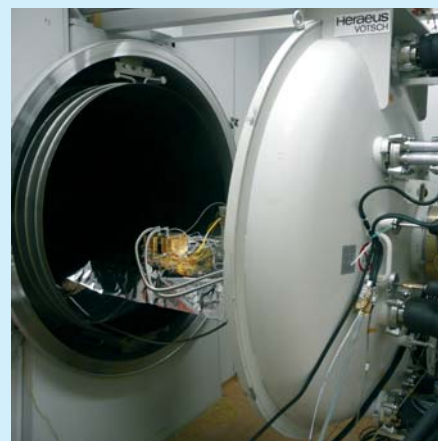
Transmitter laser assembly integrated in the thermal vacuum chamber
