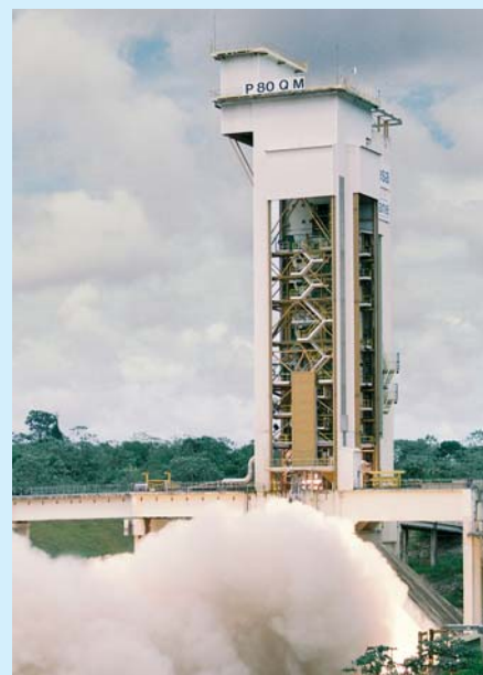
Successful P80 demonstration model firing test at Kourou
