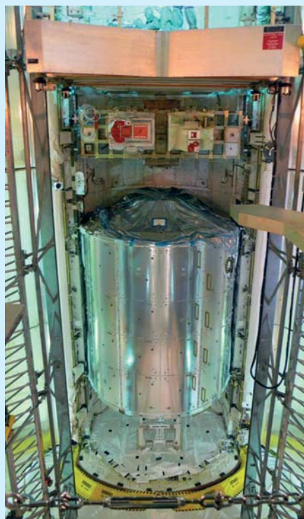
Columbus with the integrated ICC-Lite carrying the SOLAR and EuTEF payloads inside the cargo bay of Shuttle Atlantis (ESA)
