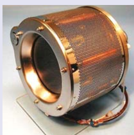
Left, ion thruster. Right, GOCE ion thruster operating at full thrust.
