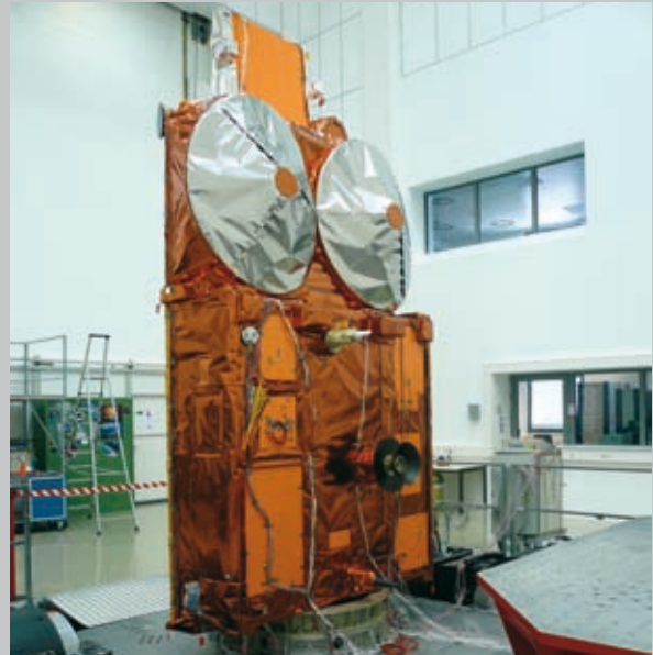
CryoSat-2 in the vibration test facility at IABG (Munich)
