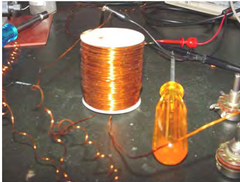
Typical John Bedini SG Bifilar Motor Coil
