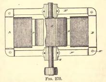
In order to secure an easier fit, the side bars EF, and end pieces, A B, are so cast that slots M are formed when the two parts are put together.
