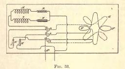
short-circuited, thereby producing a number of poles on the armature, which will tend to run the speed up above the synchronous limit. When such limit is reached or passed, the current is directed through the other coil, which, by increasing the number of armature poles, tends to maintain synchronism.
