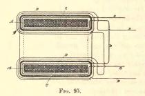
former may, by properly proportioning its several elements and determining the proper relations between the primary and secondary windings, the thickness of the magnetic shield, and other conditions, be constructed to yield a constant current at all loads.
