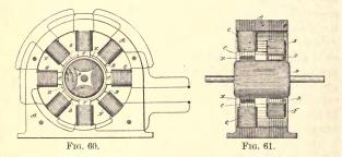
insulation between the sheets. When complete, the frame makes a field-magnet with inwardly projecting pole-pieces B and c. To adapt them to the requirements of this particular case these polepieces are out of line with one another, those marked B surrounding one end of the armature and the others, as c, the opposite end, and they are disposed alternately—that is to say, the polepieces of one set occur in line with the spaces between those of the other sets.
