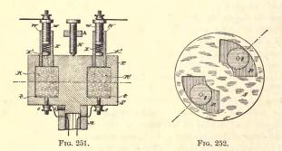
ing of the parts. In this modification the commutator and collector are made in substantially the same manner as previously described, except that the bands **B** o are omitted. The four segments of each part, however, are secured to their respective sleeves by screws g' g', and one edge of each segment is cut away, so that small plates  $a \ b$  may be slipped into the spaces thus formed. Of
