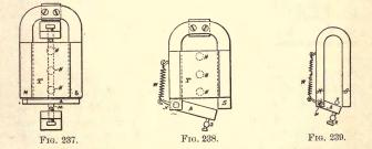
powerfully attracted and drawn into line, or nearly so, with the poles x s. In so doing the cock 6 is nearly closed and the plate T cools, the lines of force are again deflected over the same, the attraction exerted upon the armature A is diminished, and the spring w pulls the same away from the magnet into the position shown by full lines, and the operations are repeated. The ar-
