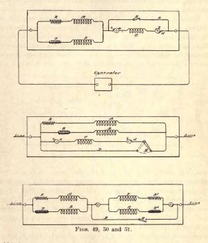
self-induction coil s in circuit with B. The same result may of course be secured by the winding of the coils. c is the armature circuit, the terminals of which are rings a b. Brushes c d bear on these rings and connect with the line and field circuits. D is the shunt or short circuit around the armature. E is the switch in the shunt.
