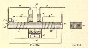
plete apparatus and Fig. 243 is a cross-section of the magnetic armature-core of the generator.
