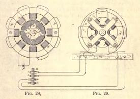
magnetic poles at all times, the rotation of the two will be synchronous; but if the motor-coils produce but six poles, the movable element will be rotated twice while the generator rotates once; or if the motor have four poles, its rotation will be three times as fast as that of the generator.
