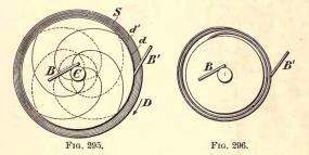
dicated by the dotted lines, the current generated will tend to weaken the magnet. In the former case the machine will be capable of exciting itself when the disc is rotated in the direction of arrow D; in the latter case the direction of rotation must be reversed. Two such discs may be combined, however, as indicated, the two discs rotating in opposite fields, and in the same or opposite direction.
