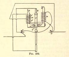
tive binding-post. Upon the passage of the current the main magnet is energized and attracts the clamping-armature g, swinging the clamp and gripping the rod by means of the gripping jaws *e.*. At the same time the armature lever L is pulled down and the carbons are separated. In pulling down the armature lever L the main magnet is assisted by the shunt-magnet N, the latter being magnetized by magnetic induction from the magnet M.
