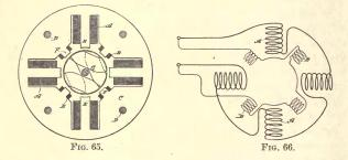
reason of the relative sizes and disposition of the cores and coils the magnetic effect of the poles E and F upon the armature closely approximate.
