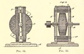
closed induced coils to intensify this effect. Although in the illustrations but one of the fields is shown, each element of the motor really constitutes a field, wound with the closed coils, the currents being induced mainly in those convolutions or coils which are parallel to the coils F F.
