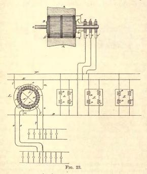
a common return-wire for both circuits, may be regarded as two independent wires. In the illustration, with the order of connection shown, coil B' of the generator is producing its maximum current and coil B its minimum; hence the current which passes through wire e, ring b, brush b', line-wire  $\mathbf{E}$ , terminal  $\mathbf{E}'$ , wire j, coils 1 1, wire or terminal  $\mathbf{D}'$ , line-wire  $\mathbf{D}$ , brush a', ring a, and wire f, fixes the polar line of the motor midway between the
