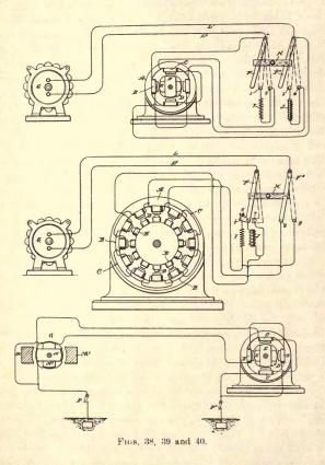
motor, the polar projections of which are wound with coils B C included in independent circuits, and D the armature with polar projections wound with coils E closed upon themselves, the motor in these respects being similar in construction to those
