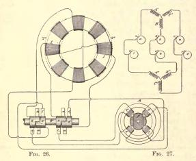
bearing on the continuous portions for taking off the alternating currents are represented by a' b' c' d'. The collecting brushes, or those which may be used to take off the direct current, are designated by M M. Two pairs of the armature coils and their commutators are shown in the figure as being utilized; but all may be utilized in a similar manner.
