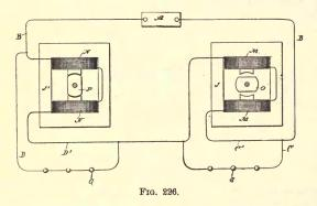
is developed in one or all of these branches of a circuit from a source of alternating currents, an active (as distinguished from a dead) resistance or opposition to the currents of one sign, for the purpose of diverting the currents of that sign through the other or another path, but permitting the currents of opposite sign to pass without substantial opposition.
